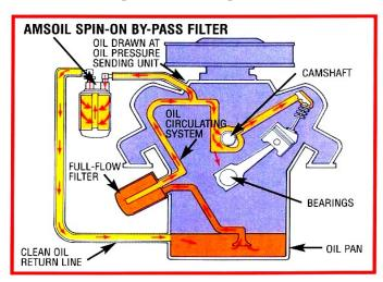
Figure 1. Typical Bypass Filter Installation (Diagram courtesy of Amsoil Corporation, Superior, Wis.)
