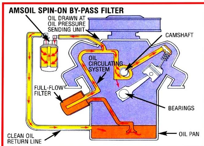
**Figure 1. Typical Bypass Filter Installation**
